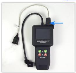
Showing the USB to RS232 adaptor with restraining clamp attached to the Surface Analyst.
