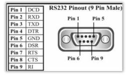
Cable length used between the Surface Analyst and the receiving equipment is limited by the baud rate selected and the capacitance of the cable used. Guidelines suggest using a baud rate of 9600 will allow cable lengths up to 500 feet.
